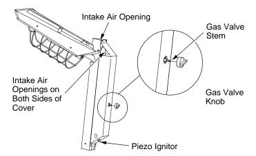
Figure 12 - Installing Gas Valve Knob
